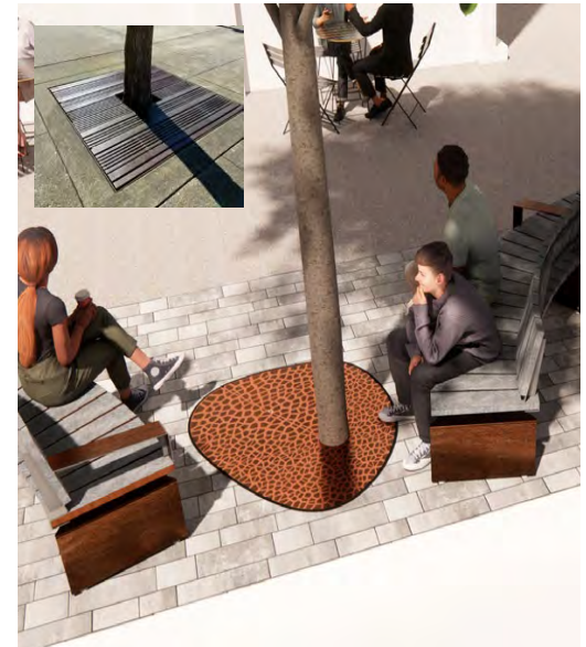
Iron Age-Custom Cast Iron Baked On Oil Tree Grate that Mimics Parasol Shape/Design-ADA accessible design with removable tree rings
