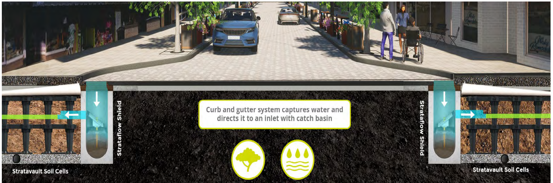
Stratavault soil cells can capture and store stormwater for irrigation, can be cut and work around existing utilities, can be left void.
