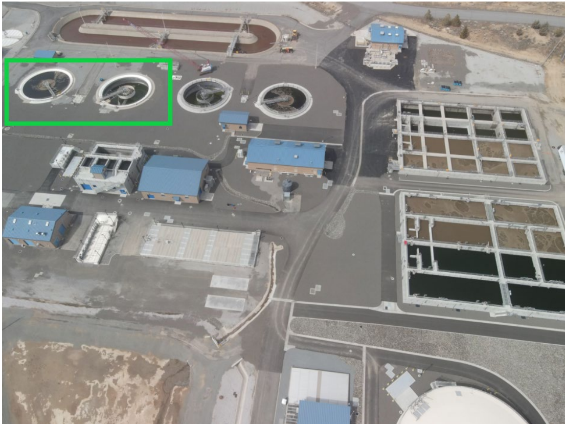
Figure 2: Secondary Clarifiers 2 & 3
