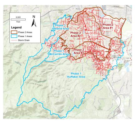
This master plan effort will expand the hydrologic and hydraulic (H&H) analysis based on the GIS platform. The Project will continue to utilize XPSWMM for the purpose of linked H&H analysis and accurate representation of flow attenuation and timing. As with Phase 1, the Phase 2 platform will be developed based on a "living model" approach to enable the master planning process to be continually updated as required.
