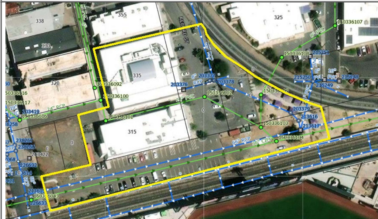
Subject Outlined in Yellow Sewer Line Easements in Green; Storm Drain Easements in Blue
