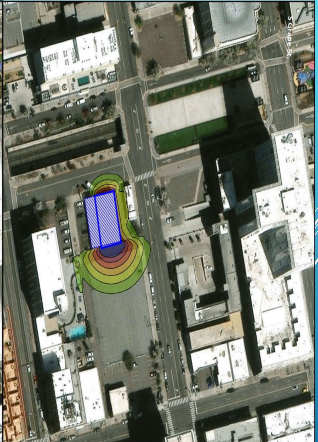
With Noise Control- 3 rd Level Interceptor
